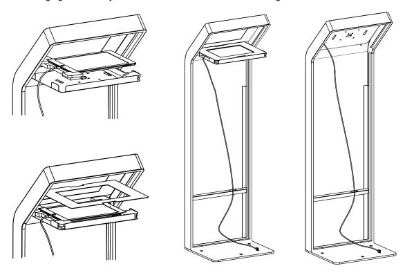
Reverse Step 1 to replace the back panel and wire the cable out through the round hole at the bottom. Lock the panel securely and the assembly is finished.
