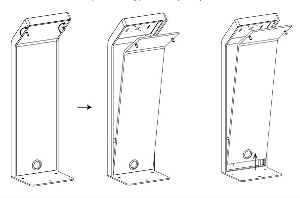
Inside the enclosure, turn the tabs outwards at the top as shown. The tablet holder can be release now.
